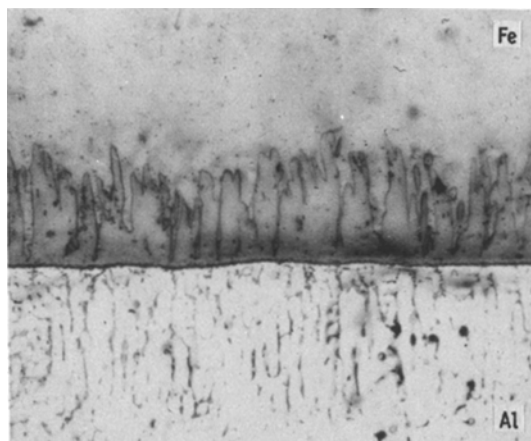
Figure 4 Micrograph of the Fe-Al interface. Temperature = 700^\circ\text{C} ; Rotation rate = 24.0 \text{ rad sec}^{-1} ; t = 250 \text{ sec} .
